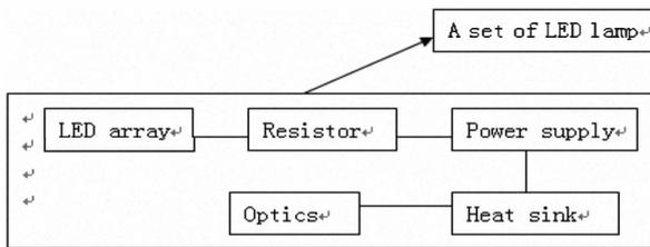
Fig.1. The structure of a LED lamp
