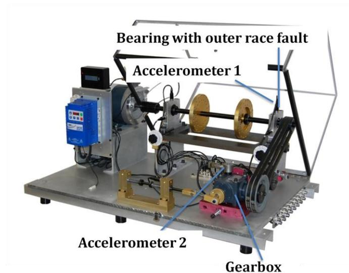
Fig. 2: Experiment setup
