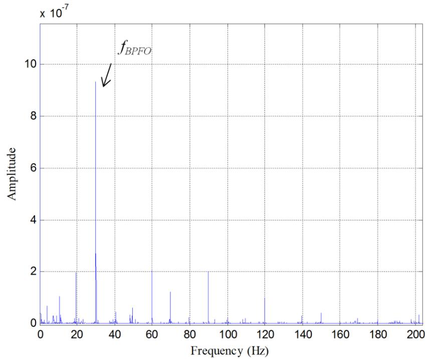
Fig.3 Envelope spectrum of the reference signal from accelerometer 1
