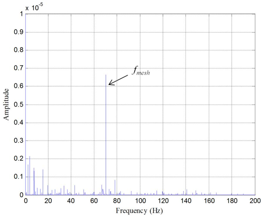
Fig.4 Envelope spectrum of the test signal from accelerometer 2
