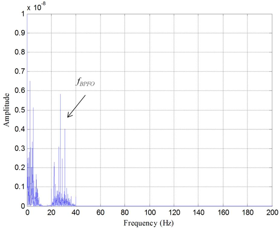
Fig.6 Spectrum of the extracted outer race fault feature using the proposed method
