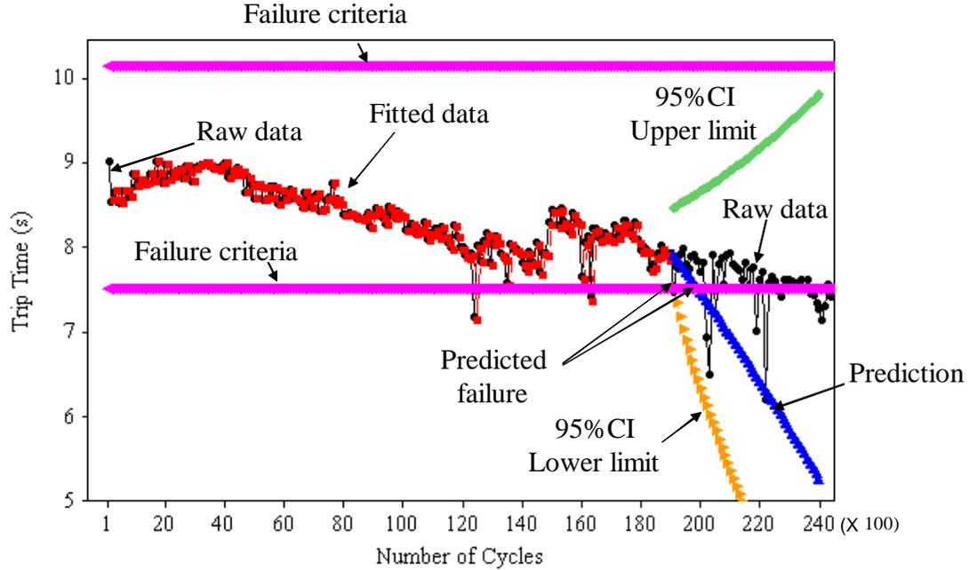
Figure 10: Prediction from the 191<sup>st</sup> to 240<sup>th</sup> points based on the previous 190 points.
