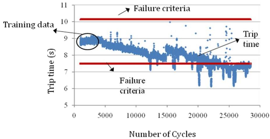
Figure 2: Trip time signals of a fuse (Sample A).
