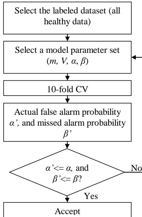
Figure 5: Model parameter selection procedure by 10-fold CV.
