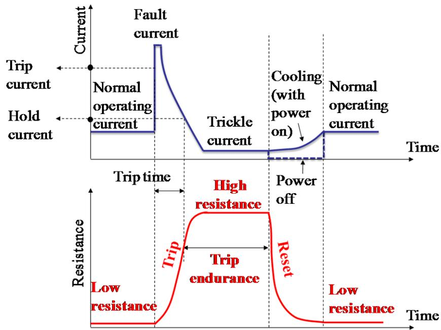
Figure 1: Operational process of resettable fuses.
