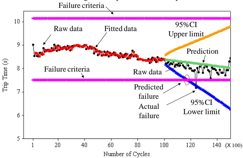
Figure 9: Prediction from the 101<sup>st</sup> to 150<sup>th</sup> points based on the previous 100 points
