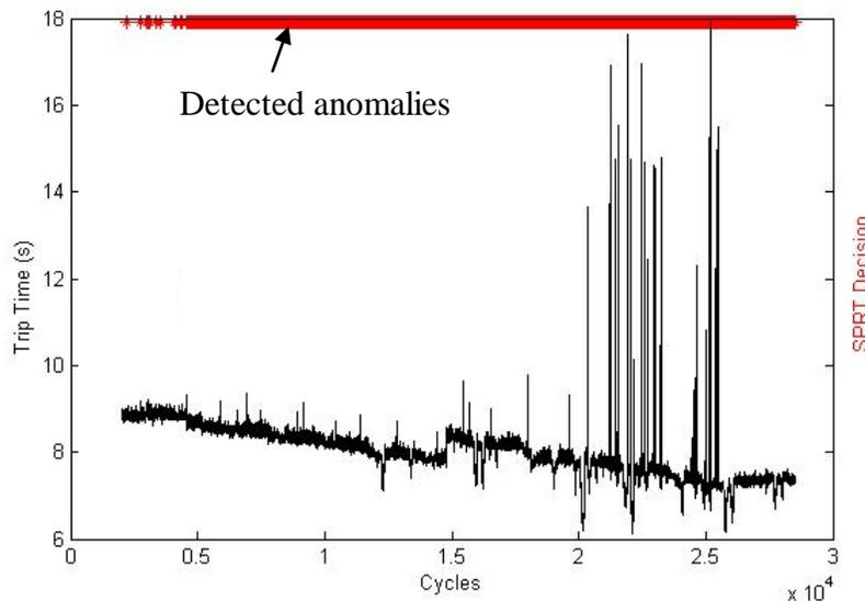
Figure 6: Anomalies detected by SPRT.
