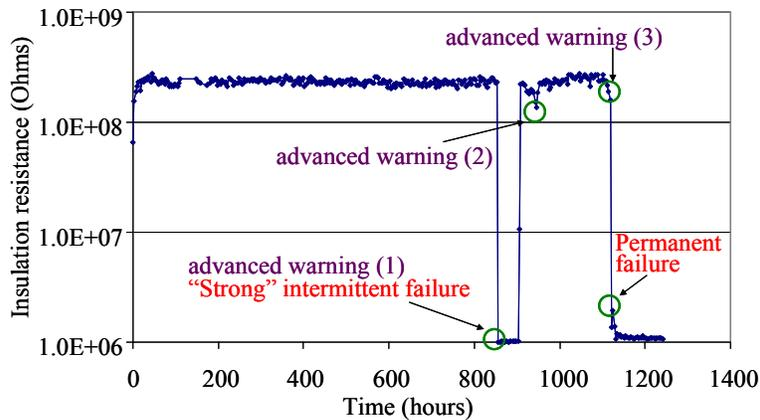
Figure 10. Original IR values recorded from capacitor #7
