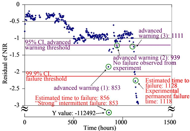
Figure 11. Residual of NIR from failed capacitor #7
