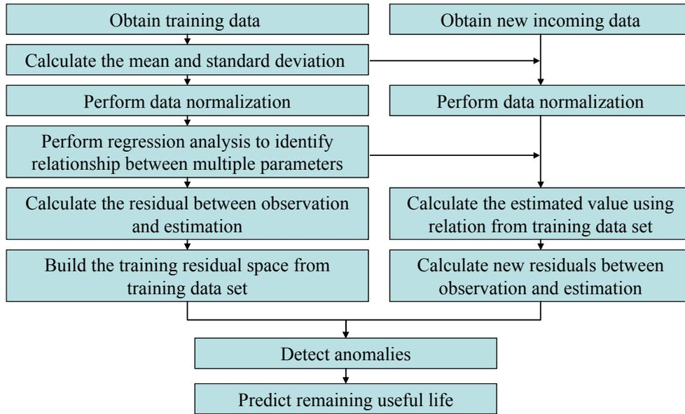
Figure 1. Regression, residual, detection and prediction analysis
