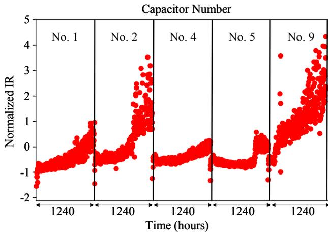
Figure 2. Normalized IR value for five survived capacitors
