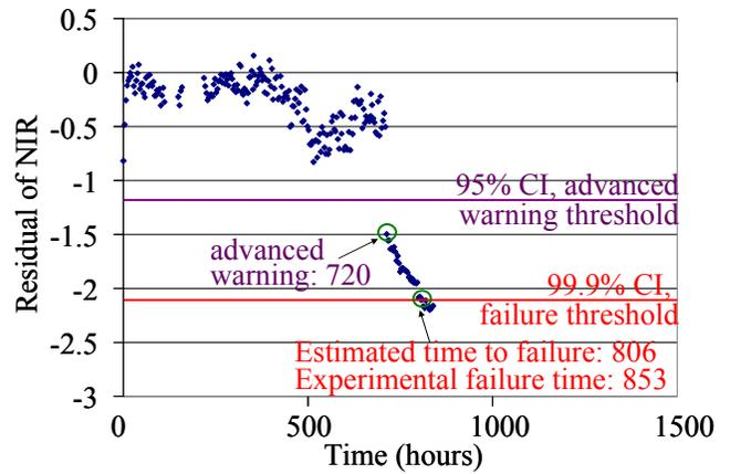
Figure 7. Residual of NIR from failed capacitor #3
