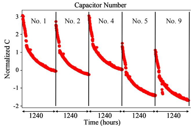
Figure 4. Normalized C value for five survived capacitors
