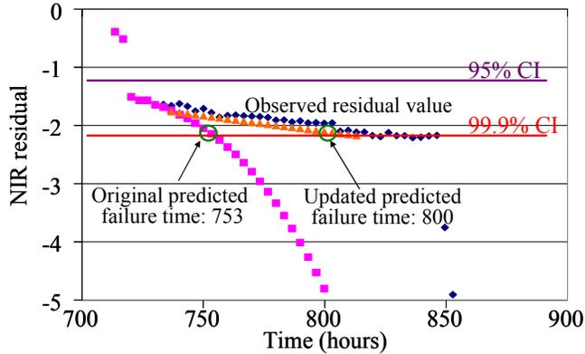
Figure 9. Prediction results for capacitor #3
