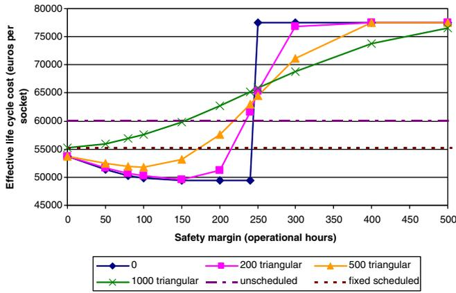
Fig. 8. Weibull distribution for the processing unit. Variation of the effective life cycle cost with the safety margin for various triangular distributions representing the LCM approach’s probability of indicating a failure. The quantities that differentiate the curves are the width of the LCM triangular distribution in operational hours. No failure outside the scope of the PHM assumed.
