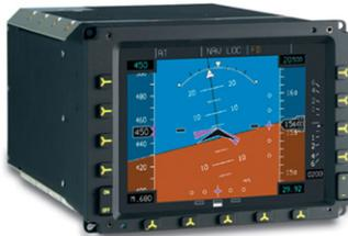
Fig. 2. Multi-function display unit (MFU).
