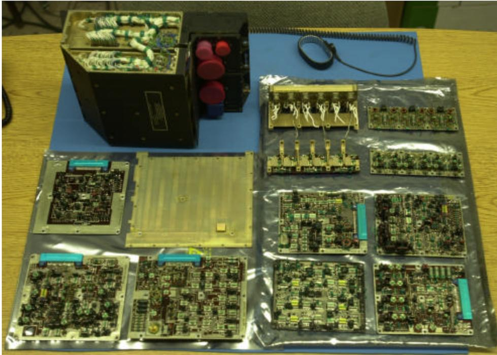
**Figure 7: Disassembled SPA unit after teardown was performed**
