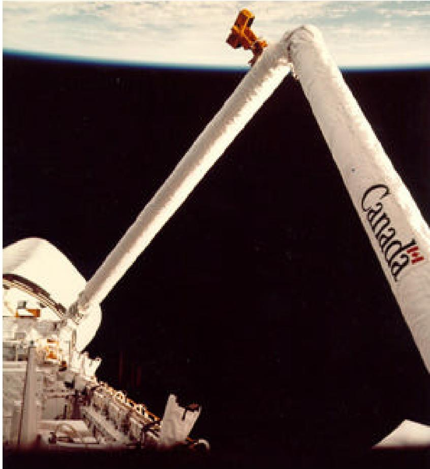
**Figure 1: Shuttle Remote Manipulator System (SRMS)**
